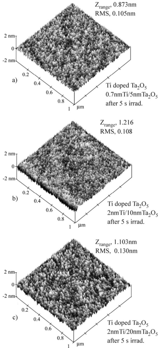
**Fig. (6).** AFM images of 5s irradiated surface-doped  $\text{Ta}_2\text{O}_5$ , with different film thickness and Ti content: a) 0.7 nm Ti/5 nm  $\text{Ta}_2\text{O}_5$ ; b) 2 nm Ti/10 nm  $\text{Ta}_2\text{O}_5$ ; c) 2 nm Ti/20 nm  $\text{Ta}_2\text{O}_5$ .
