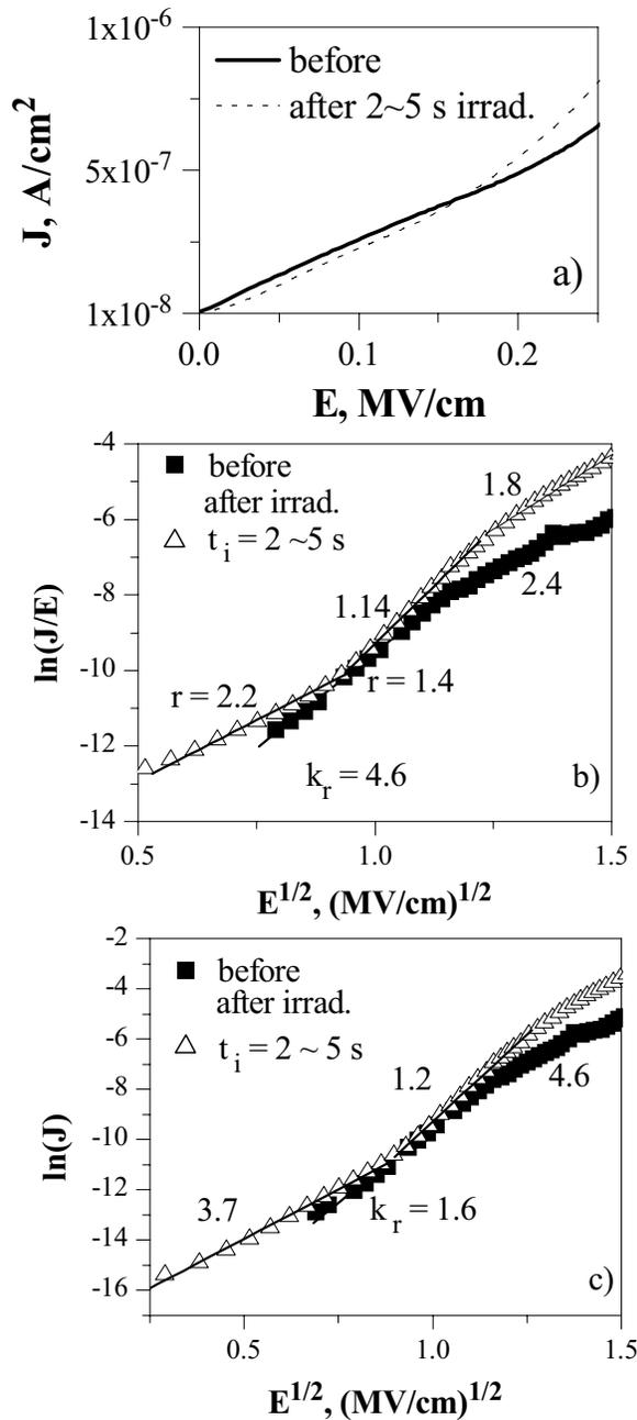
**Fig. (4).** Leakage current density of Al-gated capacitors with surface doped 2 nm Ti/8 nm Ta<sub>2</sub>O<sub>5</sub> stacked films, before and after microwave treatment in a linear scale for low field region (a); at higher electric fields in PF plot (b) and in Schottky plot (c).
