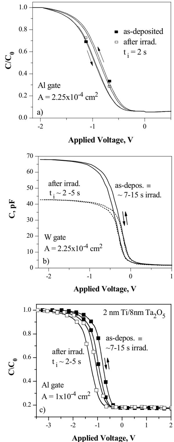
**Fig. (1).** HF C-V curves of capacitors with different Ti-doped layers before and after microwave irradiation: a) Al-gated 4 nm Ta<sub>2</sub>O<sub>5</sub>/2 nm Ti/4 nm Ta<sub>2</sub>O<sub>5</sub> stack; b) W-gated 15 nm Ta<sub>2</sub>O<sub>5</sub>/0.7 nm Ti/ 15 nm Ta<sub>2</sub>O<sub>5</sub> stack; c) Al-gated 2 nm Ti/8 nm Ta<sub>2</sub>O<sub>5</sub> stack. The arrows indicate the hysteresis direction; a) and c) normalized C-V curves.
