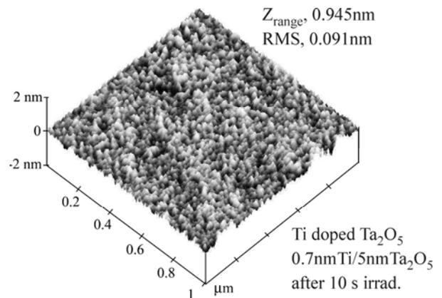
**Fig. (7).** AFM image of the surface of 0.7 nm Ti/5 nm  $\text{Ta}_2\text{O}_5$  stack after 10 s microwave treatment.
