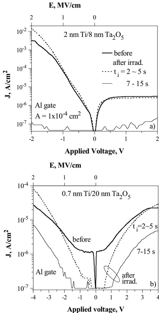
Fig. (2). Effect of microwave irradiation on the current-voltage characteristics of Al-electroded capacitors with surface doped 8 nm (a) and 20 nm (b) Ta<sub>2</sub>O<sub>5</sub> films. The gate area is 1x10<sup>-4</sup> cm<sup>2</sup>.
