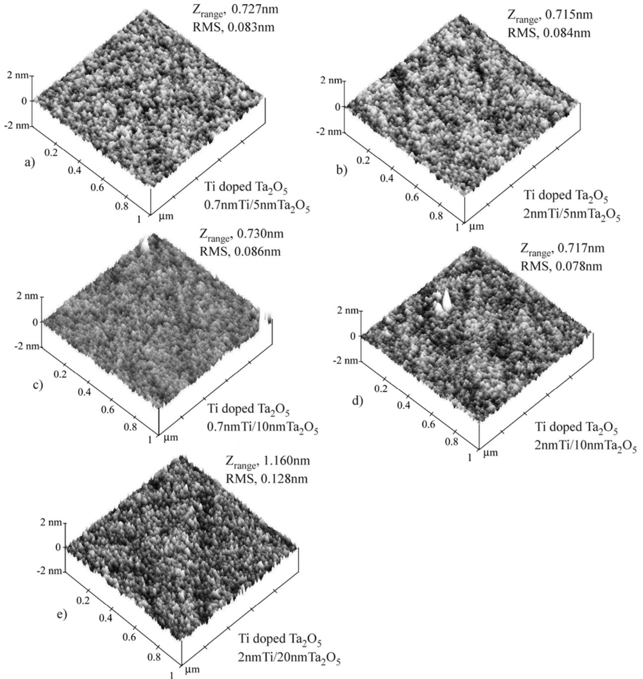
**Fig. (5).** AFM 3D topography of as-deposited pure and surface-doped Ta<sub>2</sub>O<sub>5</sub> with various film thickness and two levels of Ti doping: a) 0.7 nm Ti/5 nm Ta<sub>2</sub>O<sub>5</sub>; b) 2 nm Ti/5nm Ta<sub>2</sub>O<sub>5</sub>; c) 0.7 nm Ti/10 nm Ta<sub>2</sub>O<sub>5</sub>; d) 2 nm Ti/10 nm Ta<sub>2</sub>O<sub>5</sub>; e) 2nm Ti/20 nm Ta<sub>2</sub>O<sub>5</sub>.
